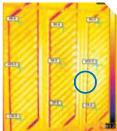
Figure 2 Hot area in a single stage setter.
