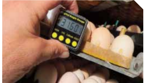
Figure 1 Turning angle of 31.6 degrees is too shallow. Target is 40-45 degrees.
