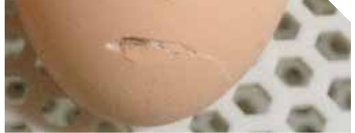
Figure 3 Damage caused by a ridge or bar on the handling equipment.
