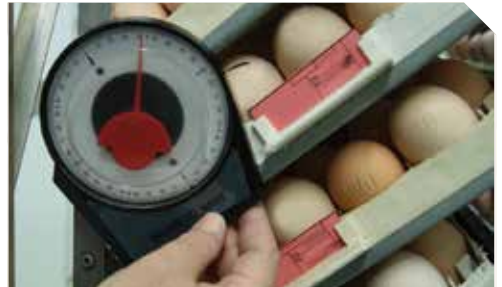
Figure 2 Getting the turning angle just right at 42 degrees.
