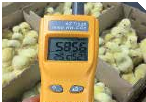
Figure 1 High CO 2 level measured in a holding room with insufficient ventilation.
