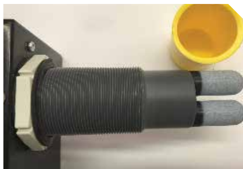
Figure 1 The photograph above shows typical CO 2 sensors in a setter, protected by sensor protection caps. If the caps become clogged with dust or condensation, the sensor will give an artificially high reading.
